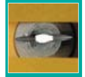
STAINLESS NOZZLE AFTER 50 HOURS
