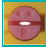
CERAMIC NOZZLE AFTER 50 HOURS
